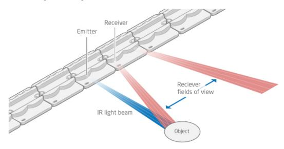
Each emitter-receiver combination covers a narrow region on the active area. An object present in the active area will affect several emitter-receiver channels, and the reported coordinates is the outcome of a center of gravity calculation on these signals.
