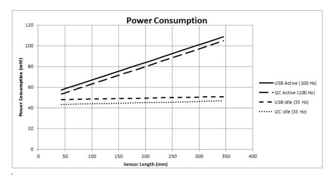
From firmware version 1.49 and higher, the sensor module types NNAMC3460PC01 and NNAMC3461PC01 are provided with Extended Range, and their power consumption increases 30% in both USB active mode and USB idle mode. The power consumption for module types shorter than 237 mm is not affected by Extended Range.
