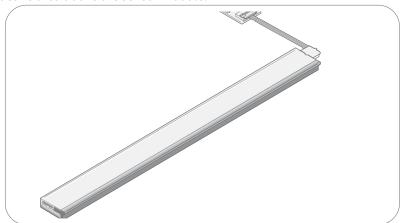
i. Alternatively, you can mount the sensor module by using tape in order to fasten the steel surface to the edge of a table, with the optical surface facing towards you.
