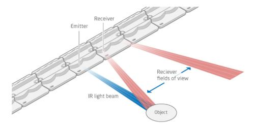
Each emitter-receiver combination covers a narrow region on the active area. An object present in the active area will affect several emitter-receiver channels, and the reported coordinates is the outcome of a center of gravity calculation on these signals.
