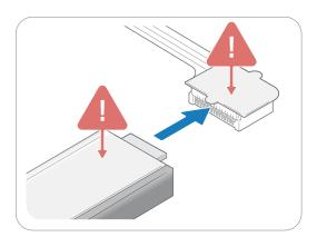
a. Place the sensor so that the sensor connector pads of the sensor are facing downwards (steel surface upwards).
