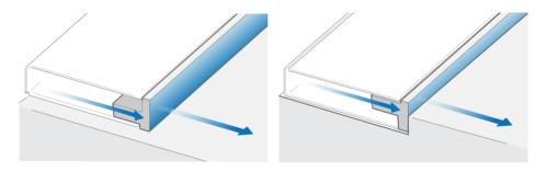
When integrating zForce AIR Touch Sensor into a host system make sure not to interfere with the light path. For horizontal integration, the opening for the sensors light path must be minimum 1.4 mm.
