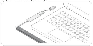
① Make sure no object is within the touch active area of the sensor before connecting power to the sensor through USB. The sensor calibrates itself when powered on and an object within the touch active area may interfere with the calibration.
