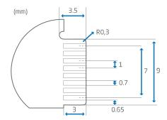
The contact pads are placed on the backside of the Touch Sensor PCBA.
