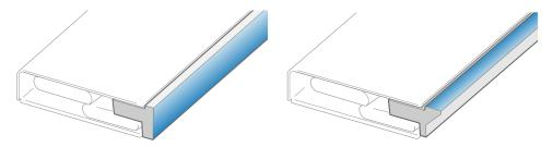
The front optical surface is not allowed to be blocked by the host system.
