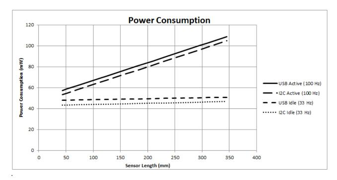
From firmware version 1.49 and higher, sensor variants NNAMC3460PC01 and NNAMC3461PC01 are provided with Extended Range, and their power consumption increases 30% in both USB active mode and USB idle mode. The power consumption for sensor variants shorter than 237 mm is not affected by Extended Range.
