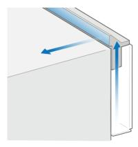
To make sure not to interfere with the sensor light path, the opening must be minimum 1.6 mm. If the host system has large tolerances, the opening must always be adjusted to be minimum 1.6 mm. Also note that it is not allowed to mount, glue or in any other way affect the sensor's optical surfaces since it will affect the performance. This applies to both the sensor's visible optical surface and the back of the mirror surface that bends the light path 90°.
